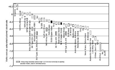
The table above gives the galvanic series in seawater. In this environment, titanium is passive and exhibits a potential of about 0.0V versus a saturated calomel reference cell which places it high on the passive or noble end of the series. For most environments, titanium will be the cathodic member of any galvanic couple. It may accelerate the corrosion of the other member of the couple, but in most cases, the titanium will be unaffected.
