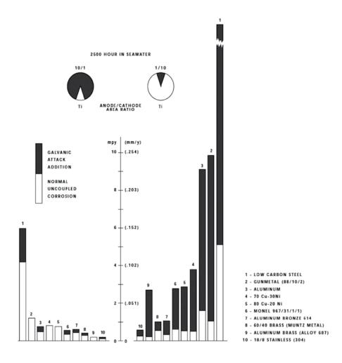
The table above shows the accelerating effect that titanium has on the corrosion rate of various metals when they are galvanically connected in seawater.
